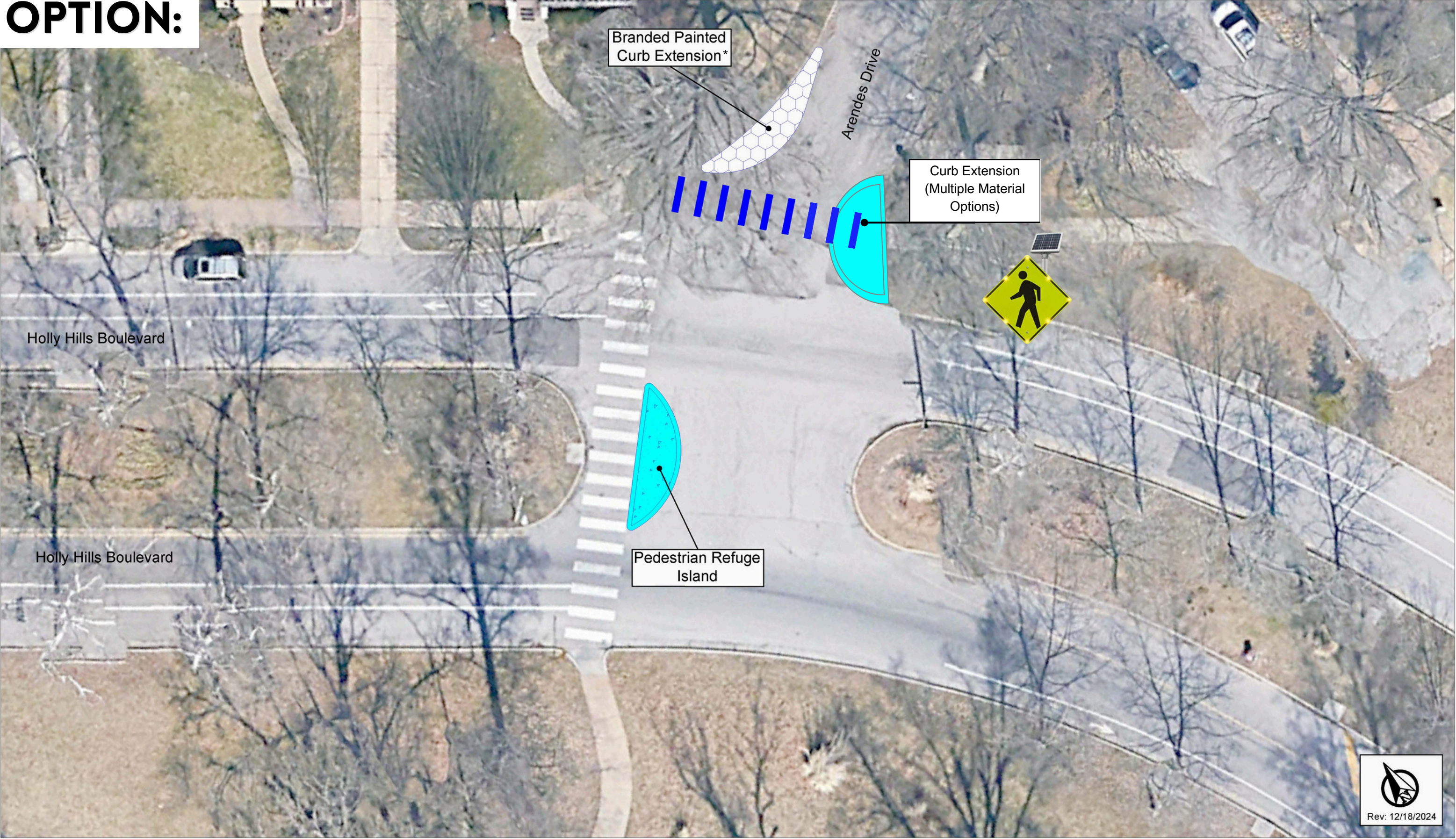
Holly Hills Boulevard and Arendes - Pedestrian Refuge Island, New Crosswalk, Painted Bumpout with Branding Cost Estimate: $10K-$20K *Painted Curb Extension could extend into interesection around crosswalk for increased visability.
